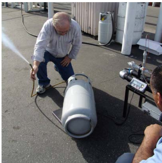
Figure 11: Liquid phase emissions measurement using scale
