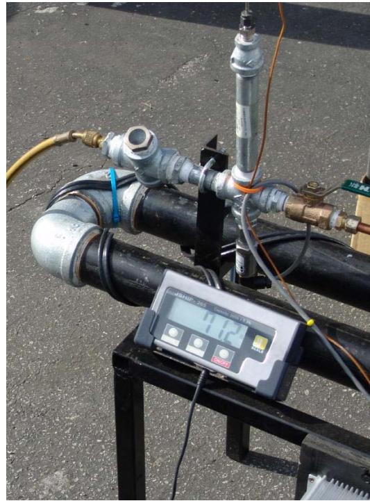
Figure 4: (a) Sight glass and instruments at gas inlet; (b) Cylinder scale display
