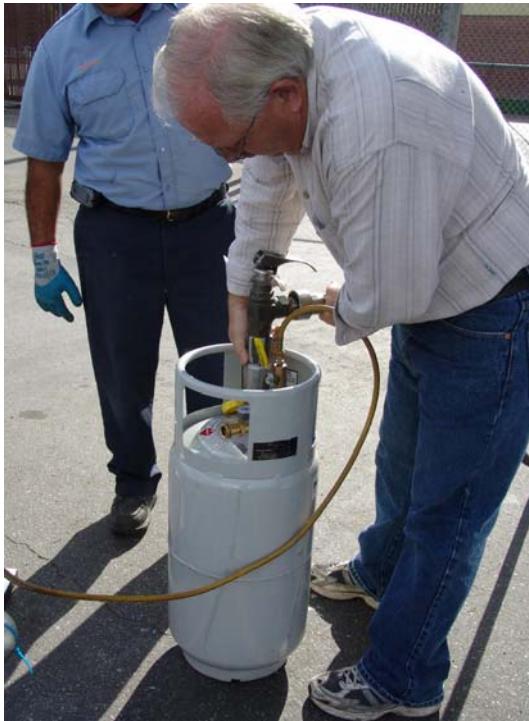
Figure 3: Connection of LP Gas source to forklift cylinder fill port
